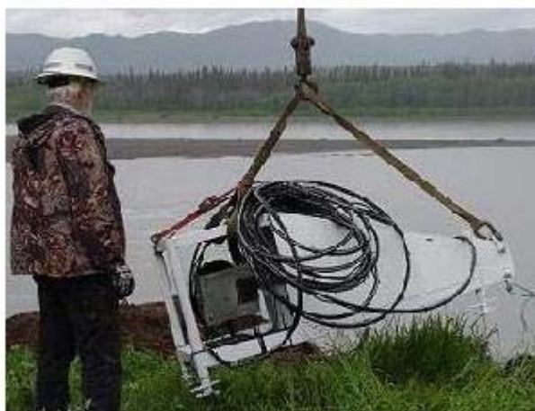
A worker watches as the transducer and housing are lowered to the bank of the Yukon River.
