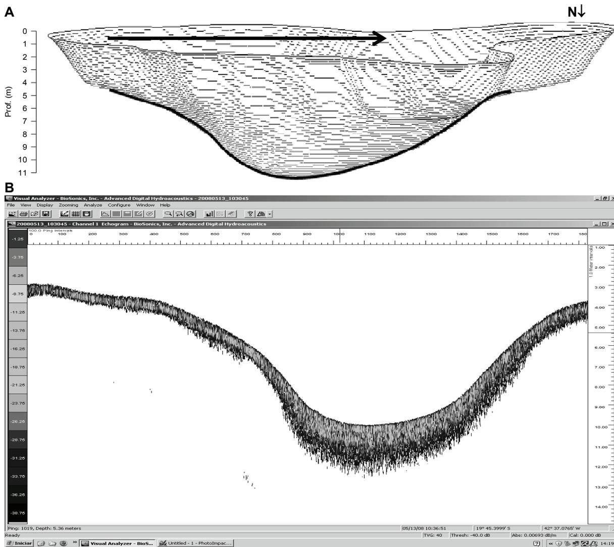
**Figure 3.** (A) Bathymetric profile in 3D view of Carioca Lake, Parque Estadual do Rio Doce, Minas Gerais (North – South view), with emphasis on the slope of the lake bottom; (B) Echogram generated by *Biosonics* echo sounder, showing the profile of the bottom transect in the east-west direction (indicated by the arrow in the figure above), made in June 2008.
